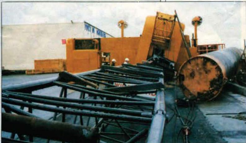
some older cranes. In other words, if a crane operator relies on the outriggers coming up to determine if he can handle the load, some part of the crane is likely to incur structural damage or total collapse before tipping occurs. This is exactly what happened in the crane accident described earlier.
